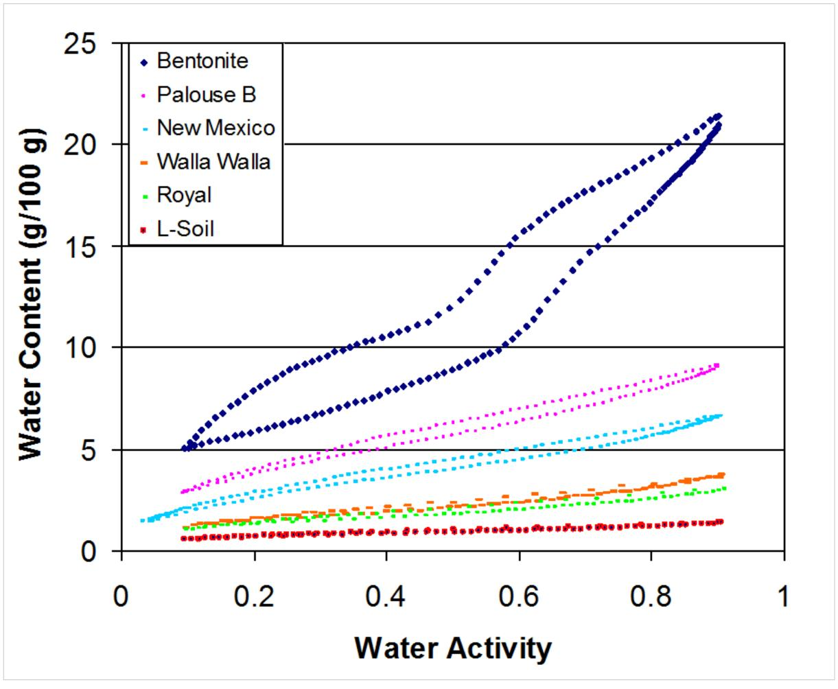
Dynamic mode: Wets or dries the sample rcontinuously in order to generate both sorption and desorption SWCCs.
