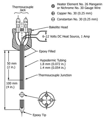
FIG. A1.1 Typical Probe Components
