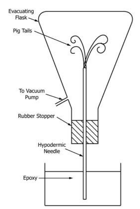
FIG. A1.2 Drawing Thermal Epoxy Into Hypodermic Tubing
