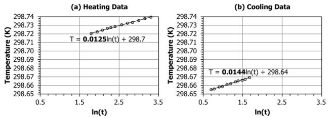
Note 1—2a shows data from the heating portion of the cycle and 2b shows data from the cooling portion of the cycle.
